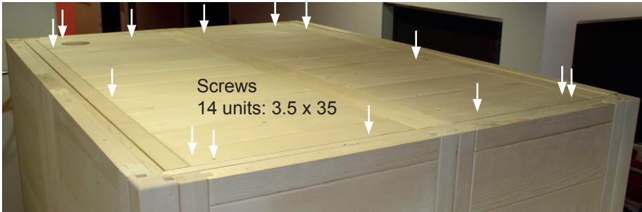
Fig. 19: Attaching the roof element
